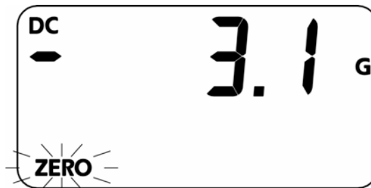
Figure 3-15 MANUAL ZERO Function
