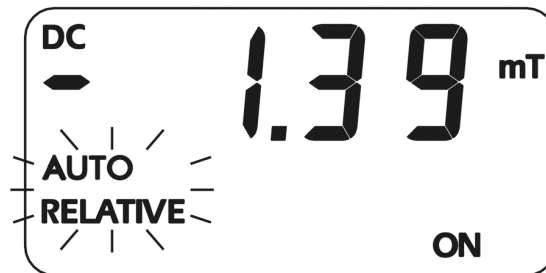
Figure 3-17 AUTOMATIC RELATIVE Function
